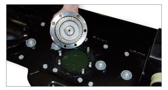
Fast and easy removal and installation of the disc bearing station for an easy and quick maintenance operation.
