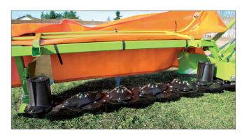
Cutter bar with low-profiled design; gears in oil bath made from high resistance steel; anti-wear skids.
