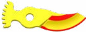
Sharpening must be done on the flat, on the 2 red slanted lines, in order to keep the same angle of penetration throughout.
