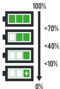
The battery charge level is indicated by the 3 LEDs on the pruning shear charge indicator. When the last LED flashes, the battery charge is less than 10%.
