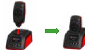
1. Place the battery (or batteries) on the charger.
