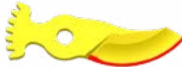
If sharpening is only done on the cutting edge, after a few sharpening operations, the fine section of the blade will disappear and you will lose the angle of penetration.
