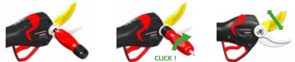
**Note:** It is possible to have a slight movement in the direction of blade closure. This movement is normal and may be caused by the gap between the rack and pinion teeth.
