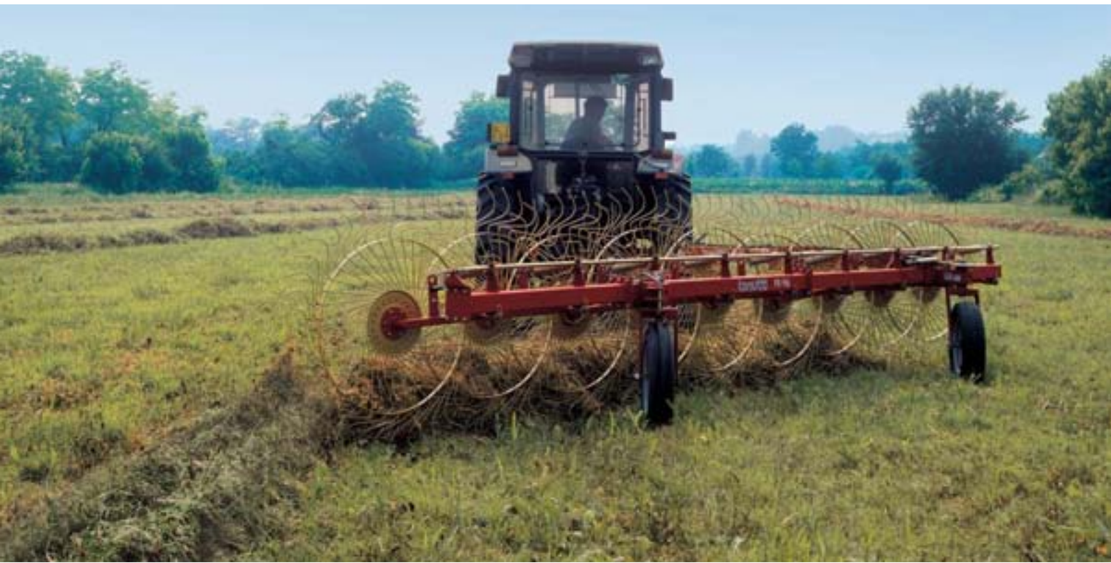
IN LINE PULL TYPE HAY RAKE mod. T 3GW with three tires
